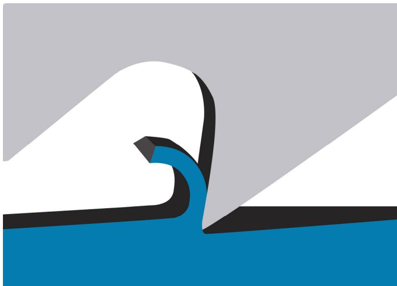
A thin cut, removing a small amount of material. Possible descent speed too slow, or blade speed too fast. Inefficient sawing.
